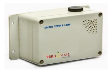
Teknovate Smart Temp & Hum is a Low Power long-range wireless radio frequency technology (LoRaWAN) based device. This highly secured data transmission technology required for Internet of Things (IoT) applications enables real-time communication of data and analytics that can be utilized to enhance efficiency and productivity.
